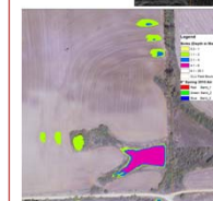
LIDAR reveals small topographic features like terrace outlets otherwise difficult to locate
