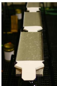
A similar setup as Study 1 was used, however, test slabs were held at a 5-degree angle from the horizontal to simulate sloped driveways and pavement in the Sacramento Valley area.
